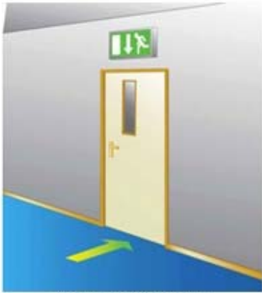
at each exit door intended to be used in an emergency
